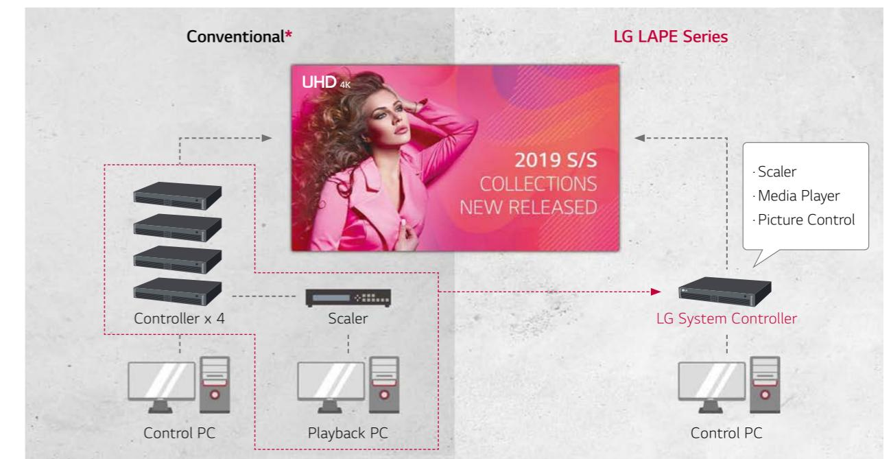
\* The "Conventional" shown above refers to LED displays that don't have an all-in-one system controller.
